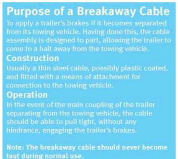
THIS ADVICE DOES NOT APPLY TO UNBRAKED TRAILERS UP TO 750kg GVW which are required by law to have the use of a SECONDARY COUPLING. A secondary coupling should keep the trailer ATTACHED to its towing vehicle even if its main coupling becomes separated.
