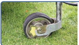
LIFT the caravan front on the jockey wheel if necessary and CHECK the noseweight
