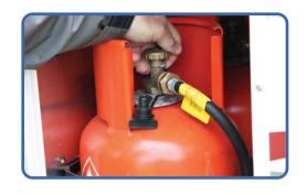
Walk all around the caravan to ensure that all the doors, windows, lockers and roof lights are closed and locked, check that any mains hook up is disconnected and the gas supply is turned off at the cylinder shut off valve.
