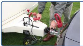
CLICK the release handle (ensure the coupling is fully on the ball) and then CONFIRM coupling engagement by raising the caravan a little using the jockey wheel,
