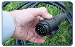
You may need an adaptor, depending upon the electrical socket(s) fitted to your car and caravan. Ensure that the cable/s at the front of the caravan are not so loose as to be able to catch or rub on the ground, nor so tight that they become taut when the car and caravan are at an extreme angle to each other. If possible, align the cable/s so that they are about 30cm (12") longer than the front of the coupling head on the caravan before attachment.
