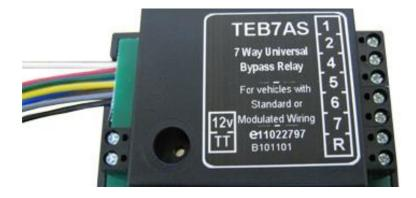
On the left hand side of the relay are 8 coloured cables, a 12v power terminal, and another terminal marked TT. The 12v power terminal requires a dedicated feed (with fuse) directly from the cars battery, while the terminal marked TT is for an optional 'tell tale' dashboard light.
