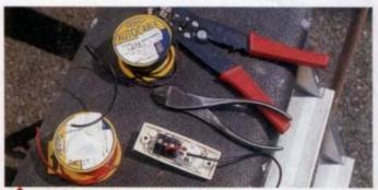
Use a short length of cable (red) to connect the output terminal of the switch to the input terminal of the neon light. A second cable (black) is connected to the output (return) terminal of the neon light. Lastly, a third cable is connected to the input – live – terminal of the switch. Both cables are then fed through the wall to the outside where the return cable is connected to the middle tube of the awning light's terminal block.
