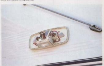
Having fitted the gasket, screw the light in position and cap the screw heads with mastic tape. You will notice that although the light has a triple terminal block, only the upper and middle tubes are used, the upper one being the supply to the switch and the middle one being the return.
