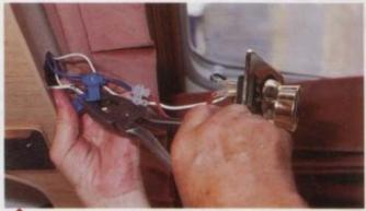
Having unscrewed the reading light, I was able to scotchlok the brown cable to the cable feeding the light's or/off switch, and the blue to the return.
