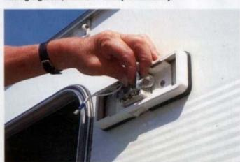
The first job is to remove the original awning light. When doing so, make sure you know which cable(s) are positive and which negative.
