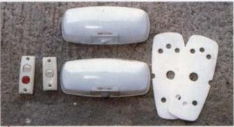
The two lights come with gaskets, so it isn't necessary to use mastic to prevent water ingress. I decided to fit an or/off switch to isolate the PIR awning light in the event of the battery's power becoming drained and when charging facilities might not be available. The illuminated switch overrides the PIR when we want the light on permanently. The light reminds us to switch off before going to bed, so we don't wake up to a flat battery!
