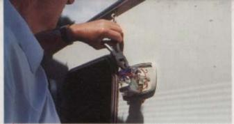
The on/off switch should now be fitted adjacent to the illuminated switch. Next, the caravan's 12v positive cable(s) are connected to a length of cable which, in turn, goes to the input terminal of the or/off switch. A second cable then connects the output terminal of the switch to the top tube of the awning light terminal block. To complete the wiring, the input cable to the illuminated switch is connected via a scotchlok to the output cable of the or/off switch.
