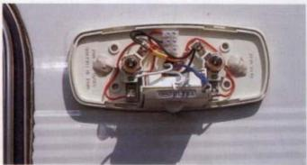
Having fitted the new light, apply mastic tape over the screw heads, again as additional protection. The light has a terminal block with three tubes. The upper one is for the power supply to the PIR; the middle one is the return; and the third – lowest – is used for the power supply, which overrides the PIR when you want the light on all the time.
