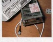
2 The CEC Plug-In-Systems Inter-Power electronic charger (above) is a single unit designed to be fitted adjacent to the battery. Its mains lead has a fail-safe plug at one end, the other being designed for connection to the van's mains supply. The 12v leads are fitted using spade connectors.
