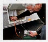
4 Having disconnected the mains power, we undid the screw at the bottom of the 6A MCB (below) and inserted and secured the brown (live) lead of the Inter-Power charger cable. The blue (return) cable was similarly connected to the return terminal and the earth cable to the earth terminal.
