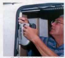
After fitting the brake light, staple the twin cable in position.
