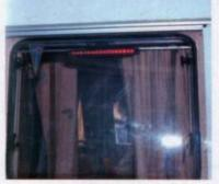
1 2 When the brake pedal is pressed, the LEDs will light up in the window to warn following traffic.
