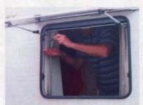
Put a prop in place to support the window and then unscrew the window stay at the inboard end.
