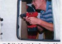
Peel back the strip from the centre of the window seal; drill a pilot hole through the frame into the wardrobe/cupboard.
