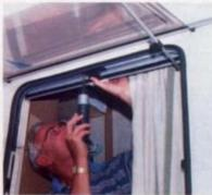
Screw the brake light bracket in position at the centre top of the window.
