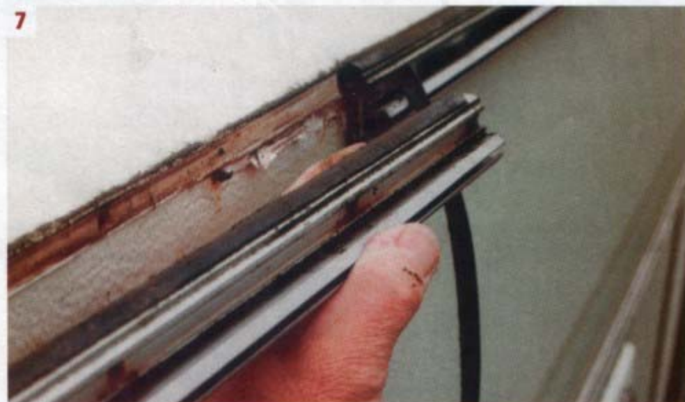
7 ■ This is a long caravan so the main section of the awning rail is joined midway along the roof
