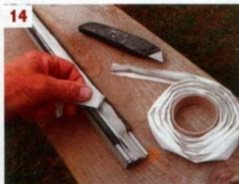
14 ■ A narrow band of ribbon sealant was pressed deeply into the moulding channels on the reverse face of the awning rail
