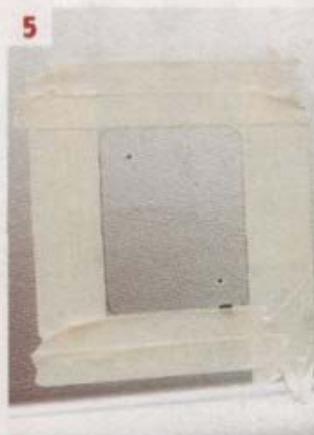
5. Masking tape protects the caravan's paintwork when cutting
