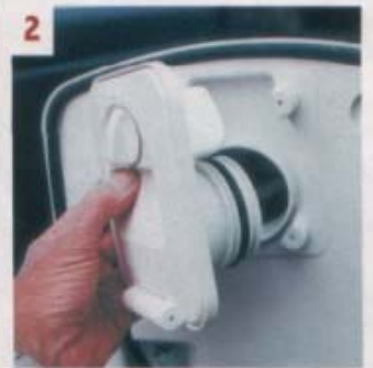
2. Ensure the filler hatch on the outside is correctly positioned
