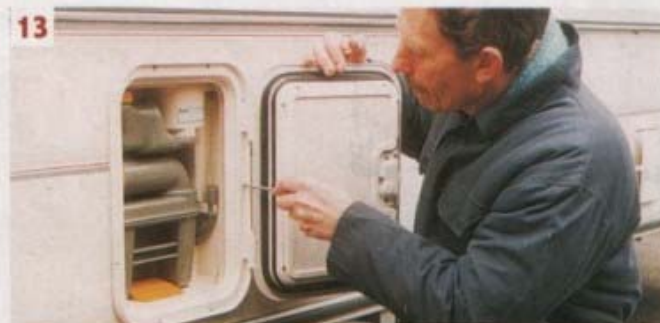
13. Make sure the hinge side of the door is nearest to the front of your caravan. Screw the toilet door in place on its bedding of sealant
