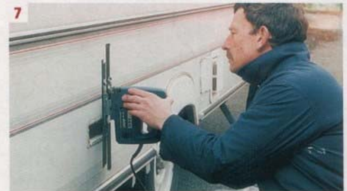
7. Carefully cut round the template border line with an electric jigsaw
