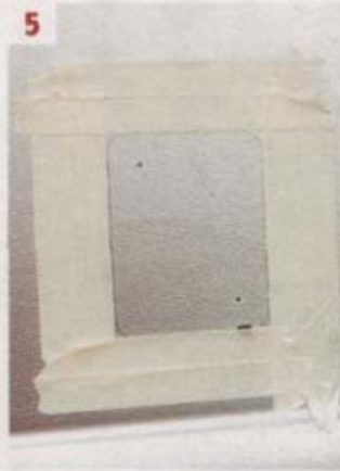
5. Masking tape protects the caravan's paintwork when cutting
