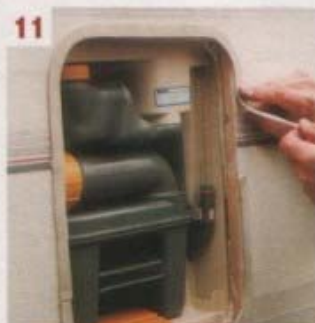
11. Ribbon sealant ensures the frame and door are water-tight
