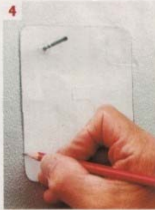
4. Draw round a template using the drill bit as a positioning guide
