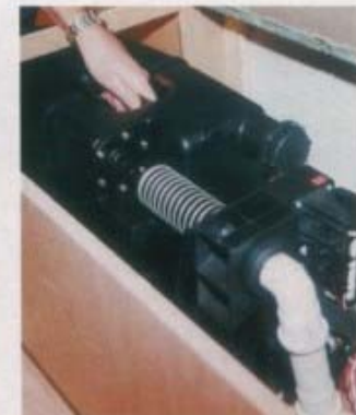
■ The vacuum mechanism and chemical-free cassette on Dometic's new product can be mounted in a bed box if required
