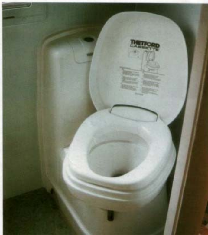
■ Swivel bowl models take up less floor space which is very helpful when a toilet cubicle's being designed
