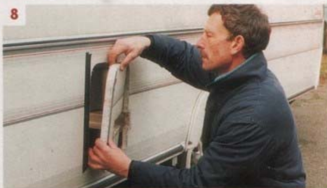
8. The section of sidewall removed needs to be kept safe for later installation within the frame of the cassette toilet access door
