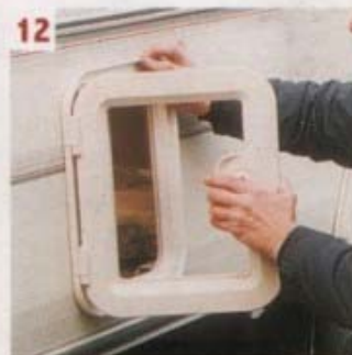
12. Doors opening this way round could blow open in the slip stream
