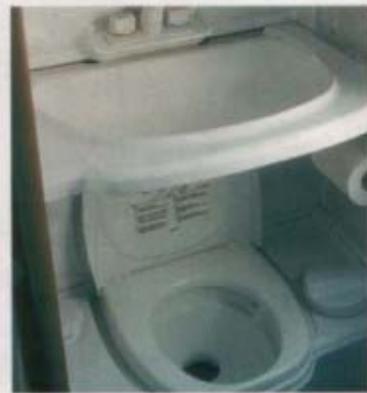
■ Where space is limited, a Thetford 'bench-style' toilet is often mounted below a lift-up wash basin
