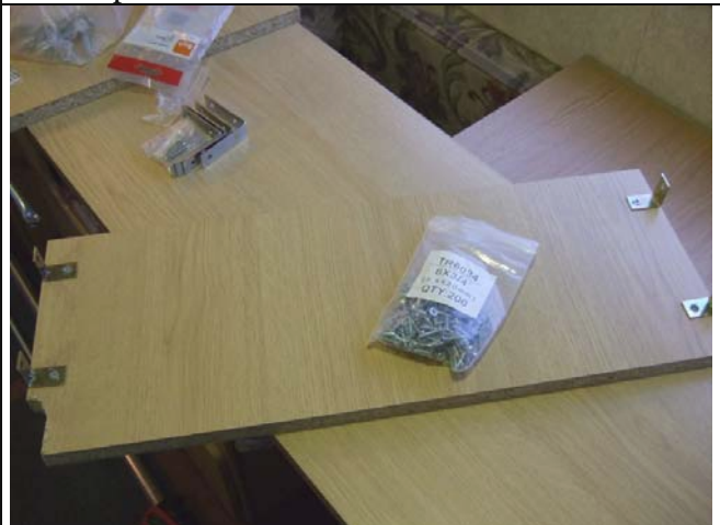
The reinforcing plinth. This is laid at the bottom of the cupboard, and secured to the side walls. It serves two purposes, it brings the bottom of the cupboard up to the lip level & it strengthens and stiffens the cupboard.
