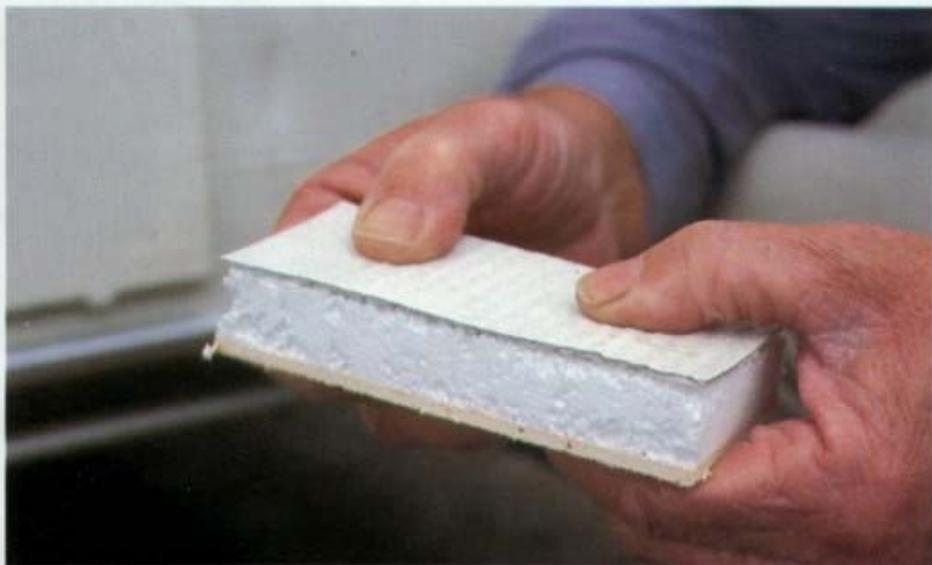
Sandwich break: wood, aluminium and polystyrene are the key ingredients of a typical sandwich-construction caravan wall
