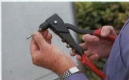
The trusty rivet gun. These rivets make for a permanent fixture whereas screws can always be removed later
