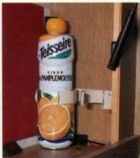
Machine screws and washers help prevent holders like this (above) from pulling through the thin interior woodwork
