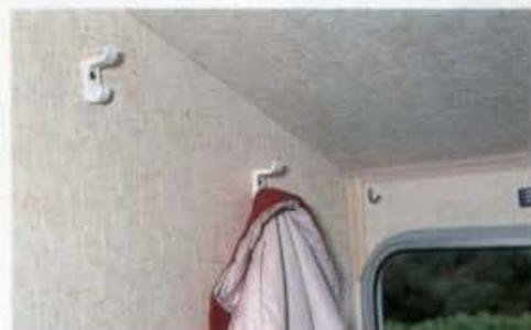
If you really must screw into an inner wall (above) it's best to use self-tapping or twin-thread coarse-thread screws
