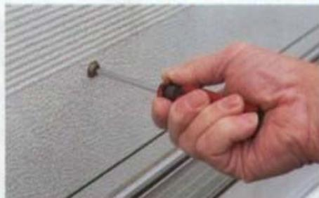
When fitting awning rail press-studs like these (above), smear a little mastic on the threads to prevent water ingress
