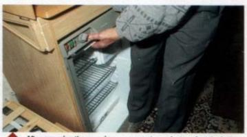
After removing the securing screws, put your foot against the hottom of the fridge and pull the fridge forward. Because the fridge sits over the wheel arch, it'll topple forward if it's not supported in this way. Once it's clear of the housing, the gas and electrical connections are accessible.
