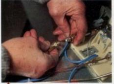
An 8mm to 8mm compression fitting needs to be fitted to the end of the gas pipe on the fridge. When fitting it, DO NOT REMOVE what appears to be a white plug in the end of the pipe. It isn't a plug, it's a filter to prevent dirt particles from reaching the burner jet.
