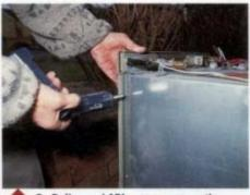
On Bailey and ABI caravans – or others where the fridge is fixed to its compartment by screws through the front trim – you will need to remove the two side trims from the original fridge and refit them to the new 4271. The screws will cut their own holes through the fridge walls.
