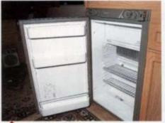
After turning off the gas and electrical supplies, the fridge can be permanently installed. At this point an extra pair of hands is a good idea – outside the caravan and through the ventilation grills to help guide the fridge into position. Finally, fit the door and grills.
