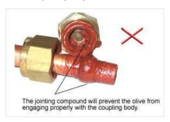
Indeed, applying a sealant could give a false impression of sealing the joint when the compression nuts may be only hand tight; also the jointing compound will prevent the olive from engaging properly with the coupling body. The resultant shrinkage of the sealant would lead to a gas leak.
