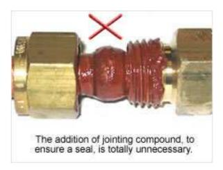
When making compression joints, Calor recommends the use of soft copper olives. These olives are easier to compress and therefore easier to produce a good seal. Brass olives, which are harder, become brittle in use and the joint can leak or fail at the point where the brass olive engages the coupling body.
