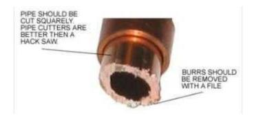
The coupling nut is slipped over the pipe followed by the copper olive. Then the pipe should be inserted into the body of the coupling ensuring that the pipe is seated firmly against the abutment shoulder. Care should be taken that the pipe does not enter the compression fitting at an angle.
