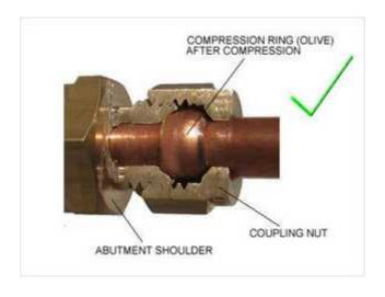
No special preparation of the tube is necessary when assembling a compression joint other than that the copper pipe is cut square and is free from burrs.
