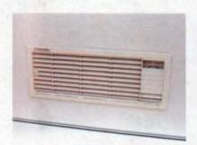
On newer caravans the fridge ventilator grilles are secured by a special locking screw.
