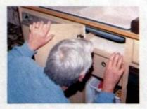
Go inside the caravan and look inside the cupboard of the unit in which the fridge is fitted. If you see light, fill the gaps with rockwool.
