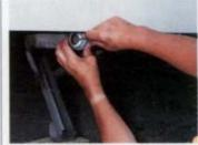
Clean the area around the steady's screw head and then fit the steady lock's outer cup over the head using a pencil or other implement to mark the position of the two holes for the high-tensile cup head setscrews.
