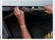
Use a centre punch and a hammer to mark the hole centres. The holes are designed to be drilled to an exact size, so take care when marking the centre – use the outer cup to check their positions before drilling.
