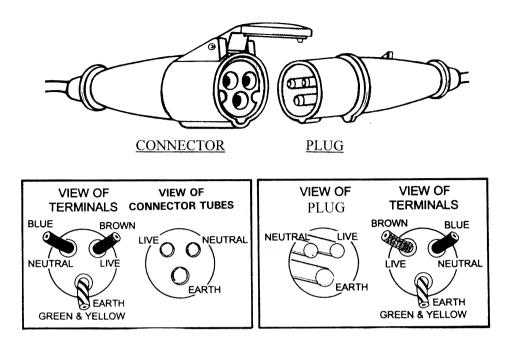
Wiring Arrangement of connector-cable
