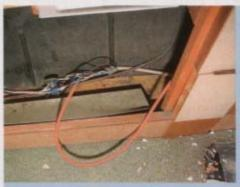
You can get some idea of the standard of wiring in the van from the state of the cables in the base of the kitchen unit. All were very light capacity and poorly connected
