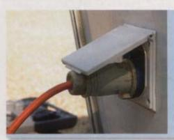
Before testing the system, I went under the caravan and made sure that the earth connction to the caravan's chassis was sound. Then I connected to the site mains
