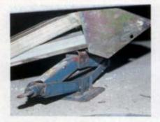
The underfloor upper plates should now be fitted between the floor and the chassis. Grease the screw and spindles of the Mule, then wind the leg down to about 40 degrees to the horizontal. Place the load spreader plate in position and use a jack to position the unit.
