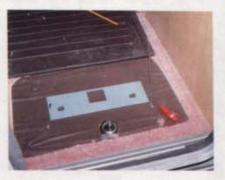
The first job is to locate the position of the chassis member by drilling a small hole up through the floor immediately adjacent to the inside of the chassis. In the illustration wire has been used to help identify the exit hole.
