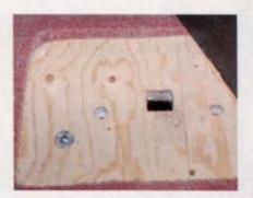
Having removed any covering over the floor, use the top plate as a template to mark the positions of the two holes for the coachbolts and the 50mm square hole. Pilot drill the floor and then drill the 25mm holes, and drill and cut the square hole.
