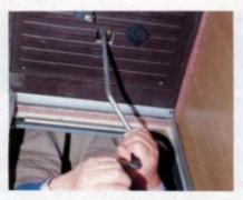
Use an open-ended spanner to tighten the shear nuts. Once the nuts are reasonably tight, use the winder to advance and retract the leg to ensure it clears the chassis. Finally, tighten the nuts until their hexagon heads shear off.
