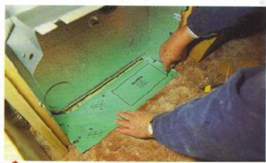
Use the paper template supplied to trim the carpet to size. You also need to decide if the heater controls are to be right-hand or left-hand mounted, as this affects the position of the floor cut-out. We chose right-hand.
