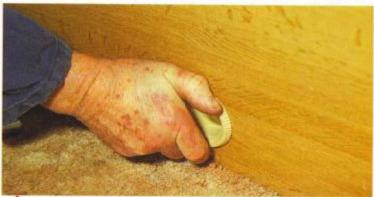
Use a 64mm hole cutter to make the holes for the blown-air outlets. The outlet nut is then put through the hole and screwed into the air outlet. Use a 70mm hole cutter to cut the holes where the ducting is to pass through partitions, seat ends etc.
