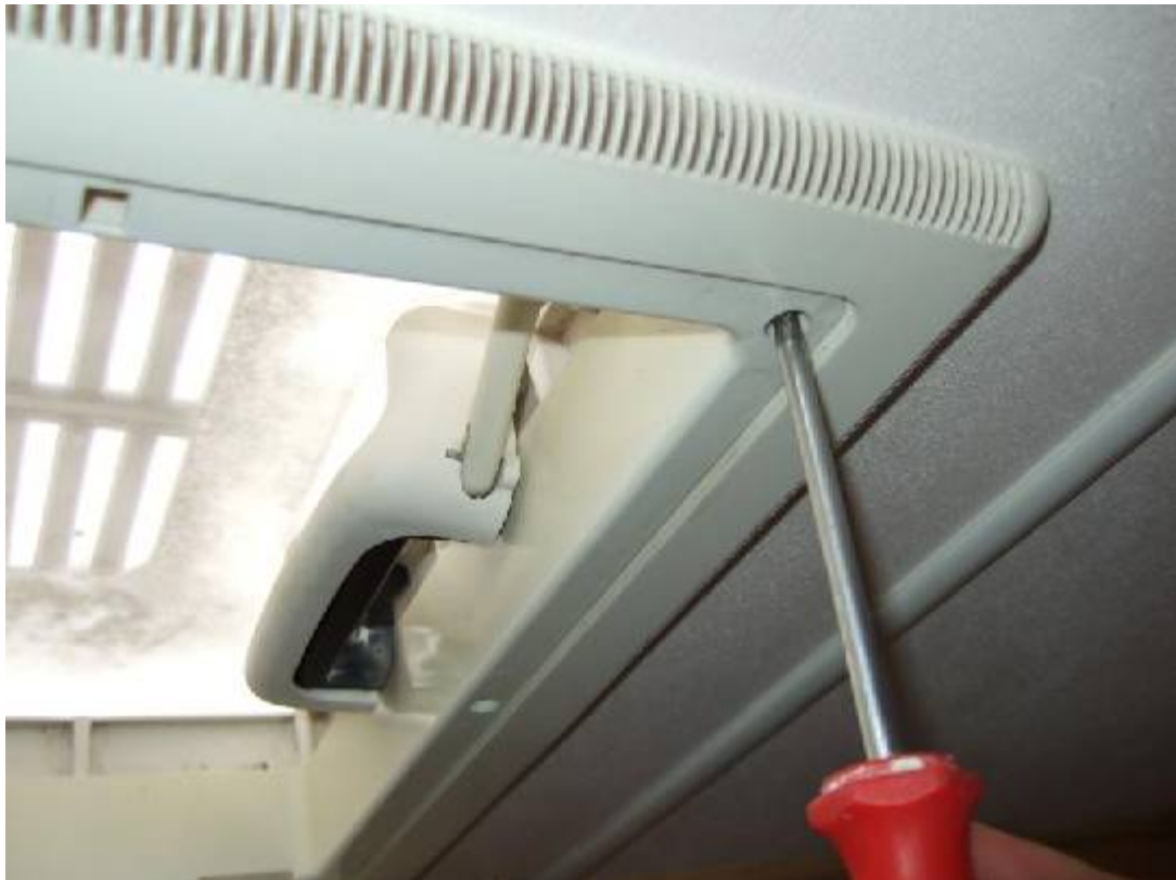
The first thing to do is unscrew the old inner surround
