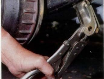
Insert the brackets into the slot in the underside of the swing arm. If necessary, use a pair of pliers to press the brackets together during this part of the operation.
