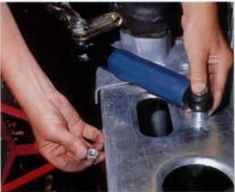
Refer to the diagrams on the carton and, if necessary, use a tape measure to confirm which one of the holes in the chassis is to be used. Insert the top bolt through the hole and fit the nut, again leaving it loose.
