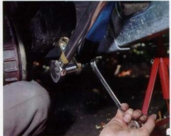
Having set the wrench to the correct torque, tighten the top nut. Align the shock absorber and the mounting bracket and then tighten the bottom nut to 86Nm (63.5 lb/ft). The nuts, incidentally, are self-locking to prevent them coming loose.
