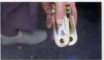
The mounting brackets are right- or left-handed and have arrows which should point forward when the brackets are fitted.
