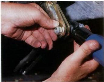
Insert the bottom shock absorber bolt through the mounting bracket. I found a pair of mole grips handy for holding the two halves of the bracket together at this point. Fit the nut but leave it loose for the time being.
