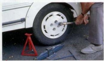
Work on one wheel at a time. Before commencing work, make sure the handbrake is fully applied and place chocks in front of – and behind – the opposite wheel. Only then should you 'crack' each stud/nut on the wheel to be removed.
