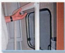
...and lifting away the complete cassette assembly. It's nice to see that Dometic have made it easy to remove and refit these units
