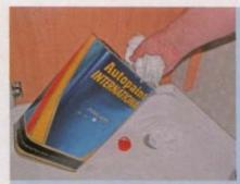
... and apply Autopaint's Panel Wipe to remove traces of grease and silicone. Apply the wipe with one cloth and wipe it off with another so you don't spread contaminants
