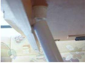
The leg should fit snugly over the bush with enough clearance from the lip of the table to allow it to fit neatly without catching on the drop spar of the table.
