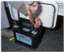
I fixed the cable to the underside of the floor with clips, using a water hose offcut to sheath it where it passed through the chassis. I drilled a hole in the battery compartment floor, fed the cable through, removed the battery, then connected up. The radio was switched on briefly to check that power was reaching it, then the battery was put back.
