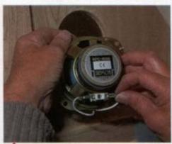
The cable pair for each channel, as supplied, has a large and a small spade connector at its end. The large one connects to the positive terminal on the speaker and the small one to the negative. If you're extending the wiring for one channel take care not to reverse this polarity or the speakers will be out of phase, which will ruin the sound quality.
