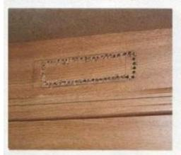
The choice of position for the radio was dictated by the position of the Status aerial booster on the Lunar. If your caravan doesn't already have an aerial, you'll have to fit one. On account of the thickness of the panelling, I had to drill holes all round the perimeter so that...
