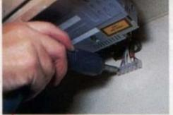
Having plugged the harness into the radio, screw the terminal block to the wall in a position where the 12v supply and speaker cables can easily be fitted. Tidy the cables so that they're not unsightly and secure them to the wall with a cable tie and saddle.
