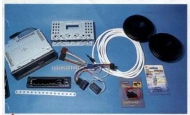
In addition to the audio unit, with mounting frame and speakers, you'll need the other items listed above — in particular, cable suitable for 12v, a length of co-ax cable and plug; and extension speaker cable (the wiring supplied will almost certainly not be long enough to reach the more distant speaker).
