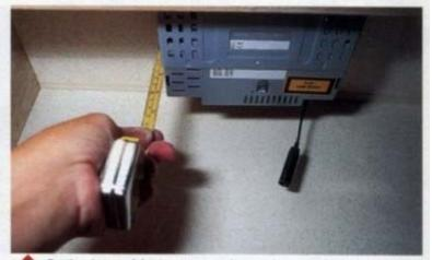
Put the player unit in place temporarily and check the distance from its top to the ceiling. The steady bracket should then be cut to length and fitted to the rear of the set as shown in the instructions, Insert the unit in the mounting frame and screw the bracket to the ceiling to secure the device in position.
