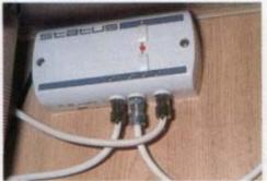
The co-ax was now plugged into one of the TV/FM terminals in the Status aerial booster. I used Superglue to hold the cable to the wall panel.
