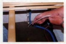
1 0 A 6mm hole was drilled down through the floor and then the cable fed up into the caravan.
