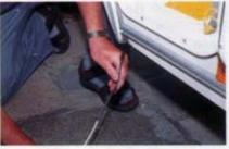
The cable was taped to a piece of coathanger wire and pushed up through the hole in the floor.
