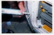
Having offered the socket and cap in place, sealant was squirted into the hole before the socket was properly fixed.
