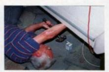
The cable was run along the underside of the caravan floor and secured with cable clips. Ensure cables don't snag.
