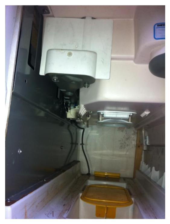
Undo the 4 pozi-screws 2 at the front 2 at the back are a bit hard to get too.
