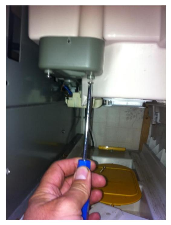
Now drop down the grey plastic bit it has the flush wiring and switches in it.
