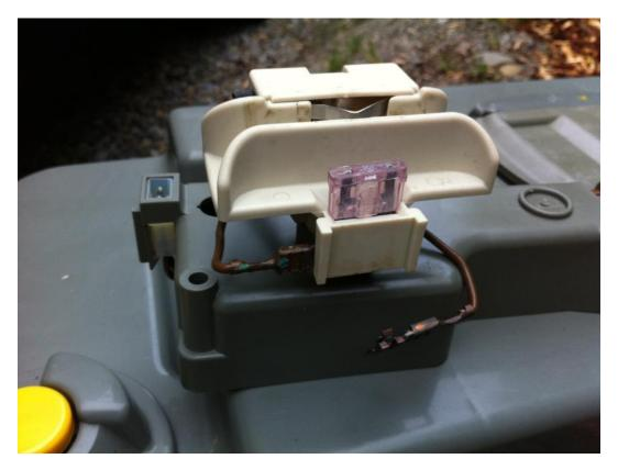
The fuse holder is so corroded it won't work. So an electrical repair to that and the whole lot can be refitted and job done!
