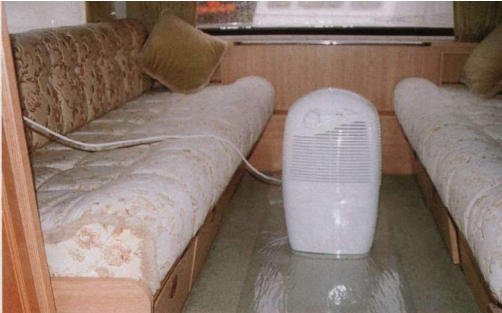
Periodically vent the caravan well. Better still, invest in a dehumidifier, which can fully dry out the structure and interior
