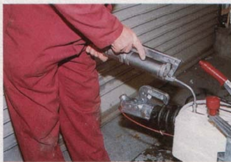
A good grease-up is worth its weight in gold over the winter. Don't forget the corner steadies and brake linkages, too
