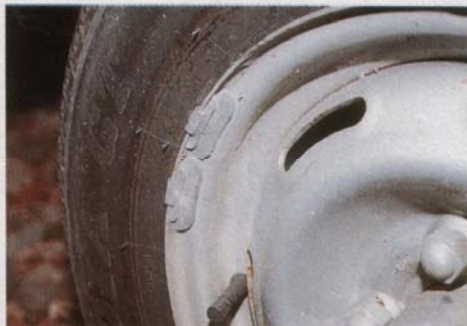
Caravan wheels need balancing as much as car ones; it makes a tremendous difference to stability and tyre life
