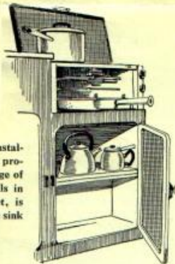
Ventilated food locker, shown above, is placed between the two single beds in the rear of the caravan. The front of this cabinet serves as a mounting for the table.
