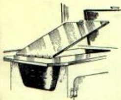
Hinged draining board cover to sink provides additional facility for food preparation.
