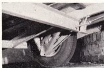
Pressed steel arms and combined coil spring and hydraulic damper units for the trailing arm suspension. Tracking adjustment for each wheel is built in
