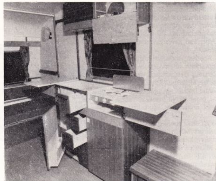
Front-end bed arrangement can be either a double or two singles; the pull-out single extensions are simple to operate and provide extra storage. Note the two drawers under the offside dinette seat
