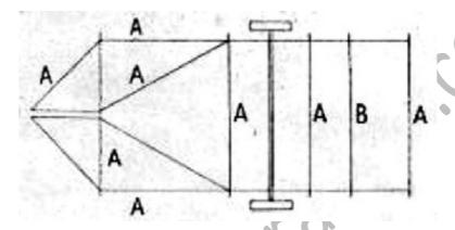
**Undergear** (sketch not to scale): A 3 x 2 x ½in, channel steel; B 2 x ¼in. angle. Box section at spring hangers, drawbar members reinforced, trusses from nose to front frame corners. Axle 1¾in. square straight. Half-elliptic springs, nine leaves, 36 x 2 x ¾in. Cam brakes, overrun cable operated. Dunlop tyres 6.50-16. Brockhouse coupling. Clamp fixing retractable jockey wheel. Brace operated legs.
